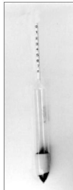
The hydrometer measures slurry density and estimates total slurry N via a regression equation (see page 6). It also provides an estimate of slurry P content.
