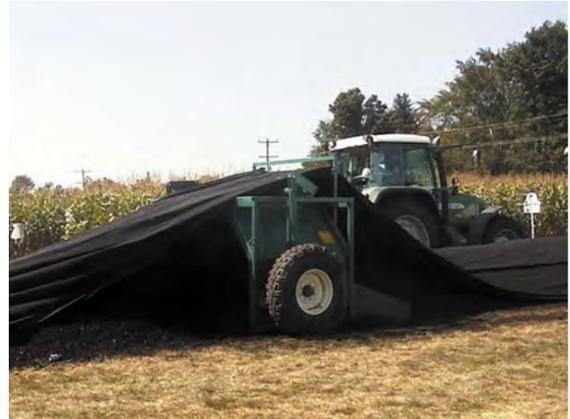
A temporary field storage of beef manure, composted in windrows, with a rain-shedding tarp that can be lifted and replaced during pile turning, has the following characteristics:
