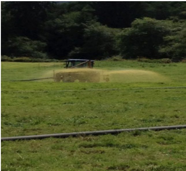
Figure 2. Place several trays, pans, or short buckets in the field to catch liquid applied with one pass with both the drag-hose application or the tank wagon.
